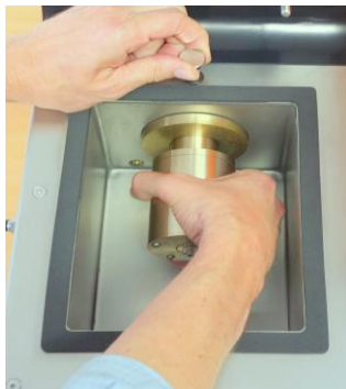
Mounting of the test-bearing housing with snap-closure arresting pin
