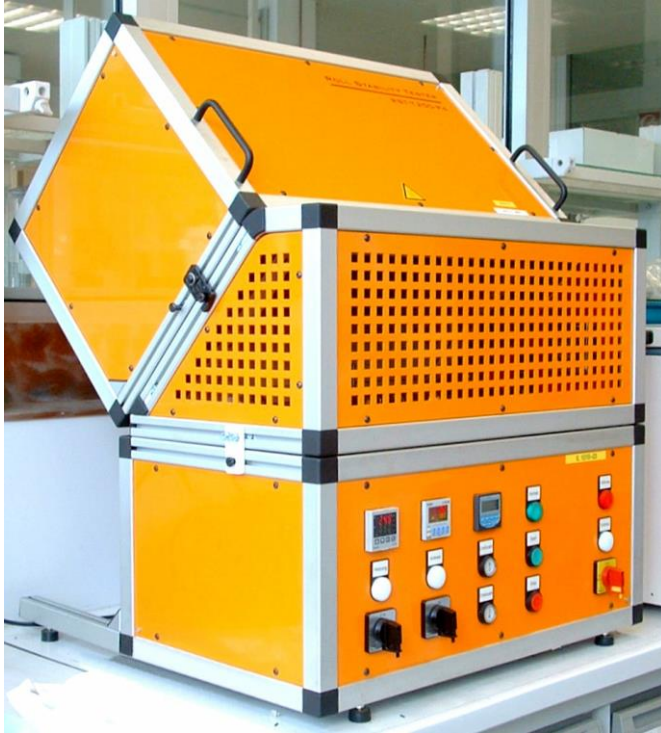
Venting hood mounted on RST
