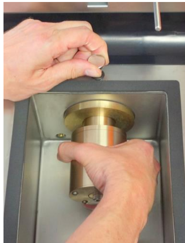
Mounting of the test-bearing housing with snap-closure arresting pin
