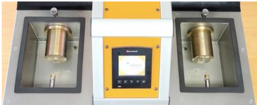
Two separate water tanks, jets and bearing housings for synchronous or independent testing
