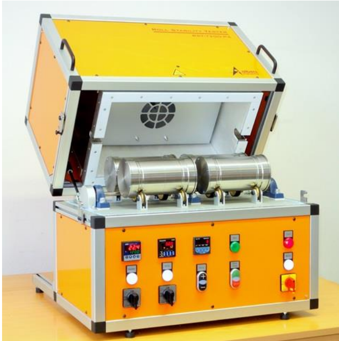
Roll Stability Tester RST-T200-P4
